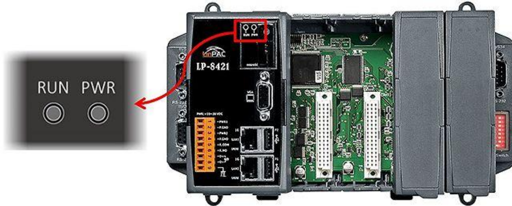
Figure 6.5.3-1. LED indicators for LP-8x2x series
